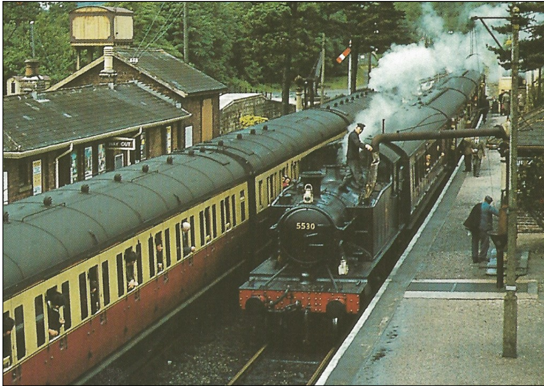
A locomotive taking water at Christow's Down platform on the last day of the passenger service. The Fireman has the "bag" in the side tank filler while the Driver operates the valve.
