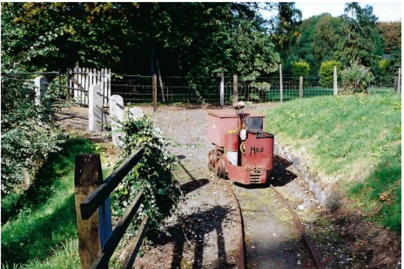
The battery-electric loco kept briefly at Christow, at 1½ tons, was far too heavy for the line. The bank to the right was cut away to allow the line to be extended.
