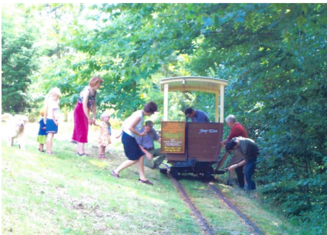
It was moved and partly rerailed before the cause of the derailment could be found. Tests later involving the car being loaded with rail chairs to destabilize it did not reveal any tendency to derail. Marks on the gauge face of the rail showed that the gear fitted to the leading axle, when it was thought that the car would be electrified, had acted to restrain it. As a precaution, the car has since always been run like this.
